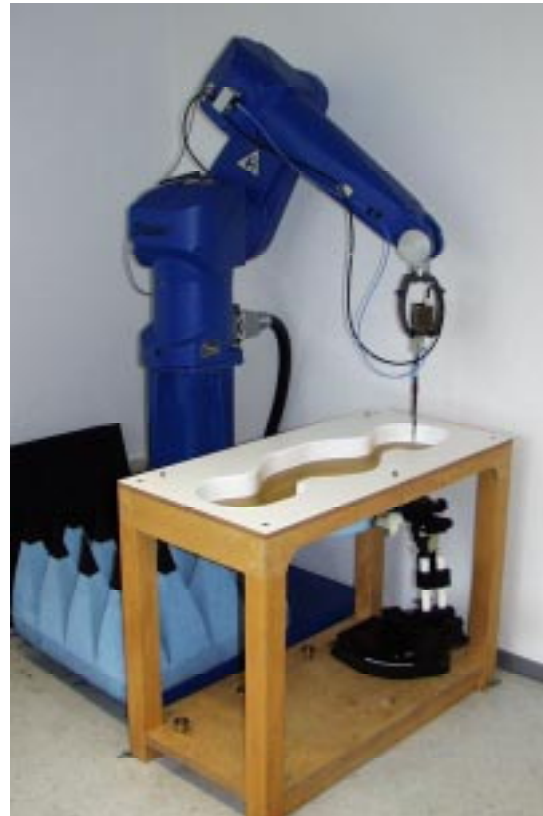
Fig. 2: The measurement setup with a phantom containing tissue simulating liquid and a MTE under test.
